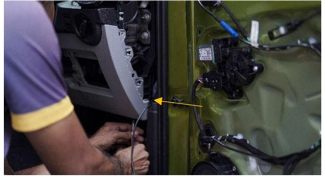
STEP 54 :- REPEAT THE SAME PROCESS ON THE RIGHT DOOR, ROUTE EXTENTION CABLE AS MARKED.
