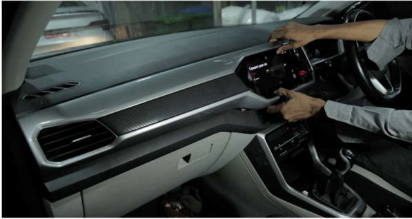
STEP 1 :- REMOVE FULL DASH BOARD PANEL AS PER THE SERIES DISASSEMBLY PROCESS
