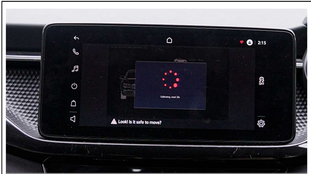
STEP 118 :- AUTO CALIBRATION WILL START, WILL TAKE AROUND 20 SECONDS.
