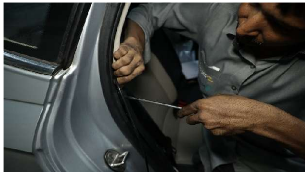
STEP 69 :- ROUTE EXTENTION CABLE YELLOW (PART 4) MALE END AS SHOWN FROM C-PILLAR
