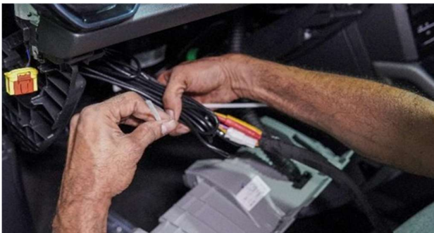
STEP 99 :- TIE ANY EXCESS CABLES WITH TIE CABLE. (PART 6)NEAR THE GLOVE BOX
