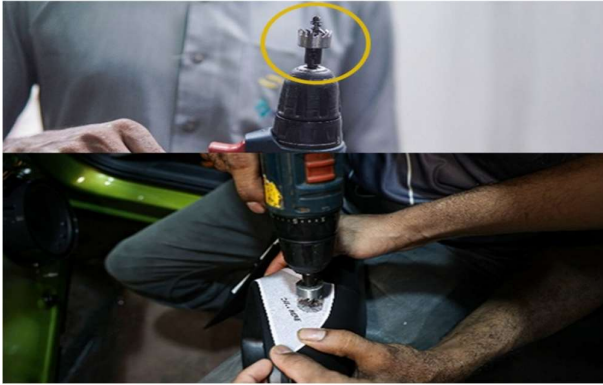
STEP 35 :- DRILL THE HOLE USING HOLE SAW 22.5 MM (PART 13) AS PER MARKINGS GIVEN ON THE TEMPLATE.
