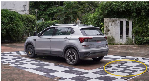
STEP 111 :- MAKE SURE THE MAT IS STRAIGHT/FLAT FROM ALL SIDES AND NOT FOLDED
