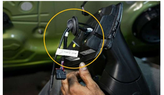
STEP 40 :- ROUTE CABLES AS SHOWN FROM RUBBER GROMMET
