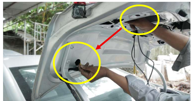
STEP 64 :- ROUTE EXTENSION CABLE YELLOW (PART 4) FROM THE BOOT AREA TO GLOVE AREA.
