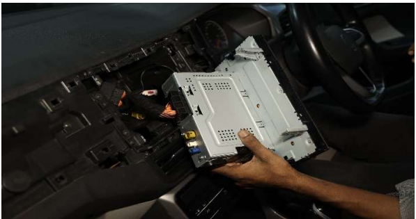
STEP 5 :- DISCONNECT ALL SERIES CABLE FROM MULTIMEDIA/INFOTAINMENT
