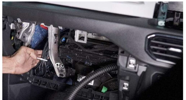
STEP 100 :- PLACE THE CABLES AS PER THE MARKED LOCATION.
