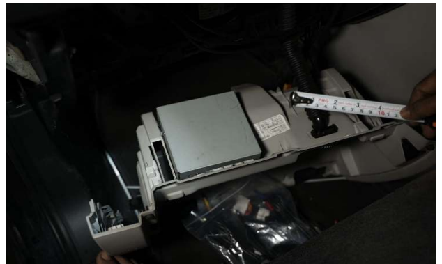
STEP 102 :- STICK THE JUNCTION BOX (PART NO 1) ON THE TOP PART OF THE GLOVE BOX.
