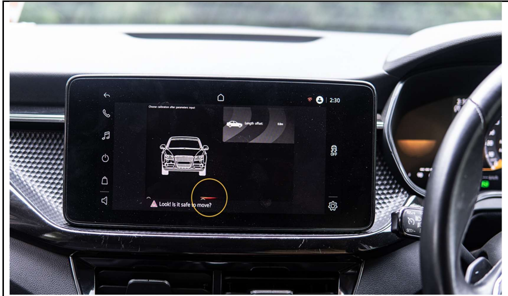
STEP 117 :- CHOOSE OFFSET AS MARKED ON STEP --,ITS 1.0 FOR VIRTUS, THEN CLICK ON "OK" AS SHOWN
