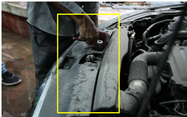
STEP 87 :- REINSTALL THE BUMPER INSERT COVER NEAR ENGINE BAY AS PER SERIES PROCESS.
