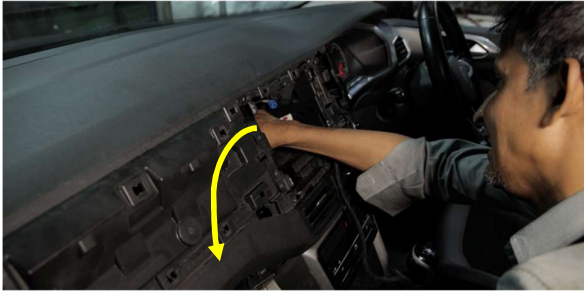
STEP 21 :- ROUTE SAVV DEDICATED POWER CABLE (PART 9 ) FROM THE BACK OF THE MULTIMEDIA/INFOTAINMENT TO THE GLOVE BOX AREA AS SHOWN
