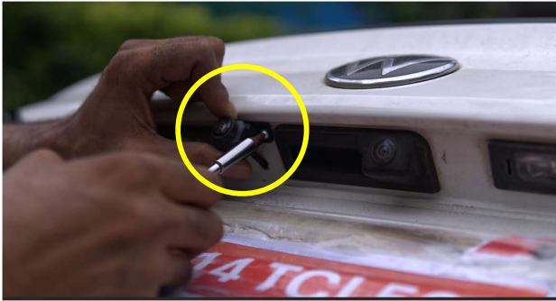
STEP 95 :- SCREW (PART NO 12) AND FIX THE REAR CAMERA. (PART NO 7). COVER THE EXTRA SPACE IF ANY LEFT FROM THE REAR CAMERA HOLE WITH THE SILICONE SEALANT PROVIDED TO PREVENT WATER INGRESS.
