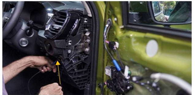
STEP 56 :- ROUTE CABLE AS SHOWN.
