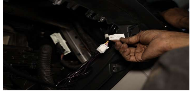
STEP 24 :- ROUTE SAVV DEDICATED POWER CABLE (PART 9 ) FROM BACK OF THE MULTIMEDIA/INFOTAINMENT TO THE GLOVE BOX AREA AS SHOWN
