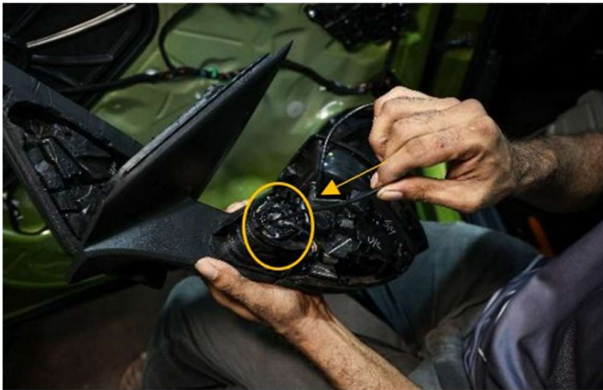
STEP 37 :- ROUTE THE CABLES THROUGH SPACE MARKED ( FOR CLEAR DEMONSTRATION KINDLY REFER TO THE INSTALLATION VIDEO)
