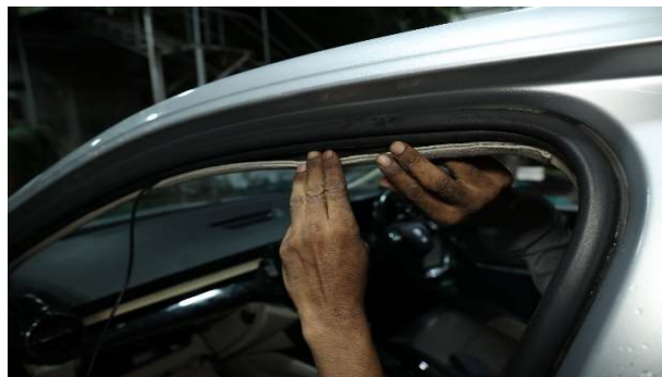
STEP 72 :- ROUTING CABLE THROUGHOUT THE ROOF LINER FROM B-PILLAR TO A-PILLAR.
