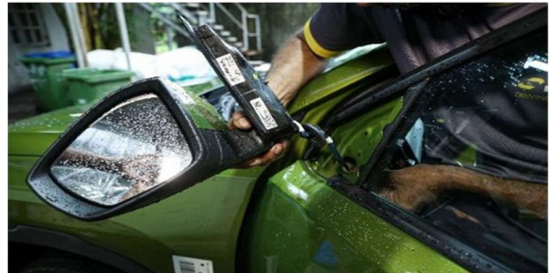
STEP 32:- REMOVE THE LEFT AND RIGHT ORVM's CAREFULLY AS PER SERIES PROCESS.
