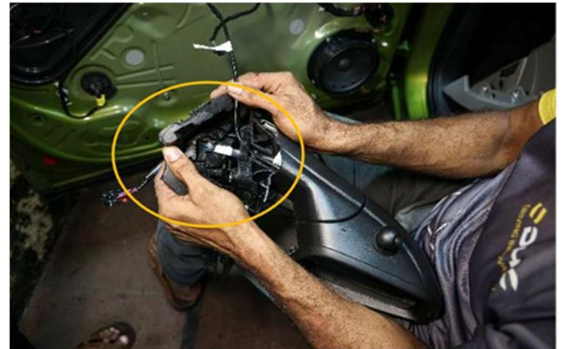
STEP 38 :- REMOVE THE FOAM PART
