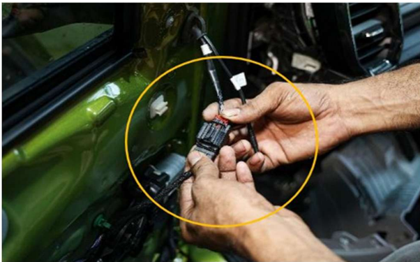
STEP 43 :- CONNECT ORVM's CONNECTOR
