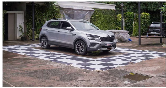
STEP 112 :- OVERVIEW OF THE MAT SETUP – EQUALLY ALIGNED ON ALL 4 SIDES (PUT SMALL WEIGHTED OBJECT ON THE MAT IN ORDER TO RESTRICT MOVEMENT OF THE MAT)
