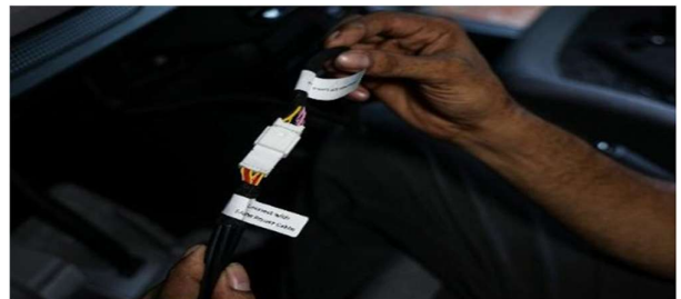
STEP 26 :- CONNECT THE 32 PIN CONTROL CORD (PART 6) WITH SAVV DEDICATED POWER CABLE (PART 9) AS STEP 10
