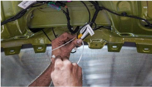
STEP 97 :- TIE ANY EXCESS CABLE WITH TIE CABLE (PART 6)
