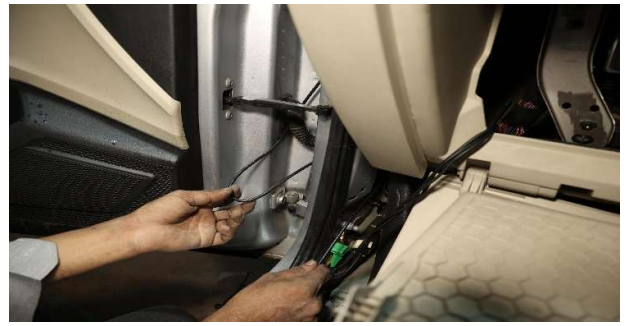
STEP 84 :- ROUTE CABLE THROUGH RUBBER SLEEVE AND THE GLOVEBOX AREA (KINDLY REFER TO THE VIDEO IF ANY CONFUSION).
