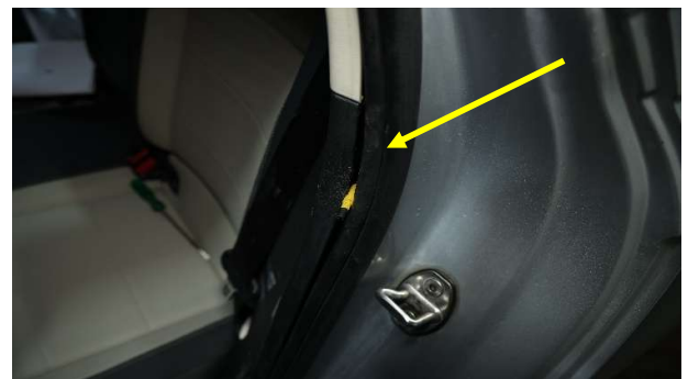
STEP 68 :- ROUTE EXTENTION CABLE YELLOW (PART 4) MALE END AS SHOWN FROM C-PILLAR
