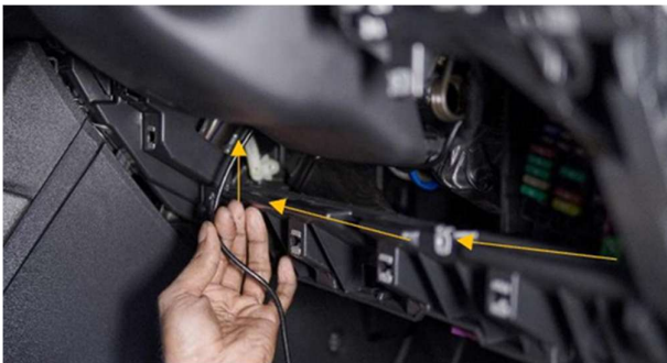
STEP 57 :- ROUTE CABLE AS SHOWN UNDERNEATH STEERING COLLUMN.
