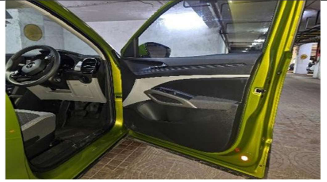
STEP 60 :- ASSEMBLE DOOR TRIM OF THE LEFT AND RIGHT DOOR + OVRM AS PER SERIES PROCESS AFTER ENSURING ALL ELECTRICAL CONNECTIONS.
