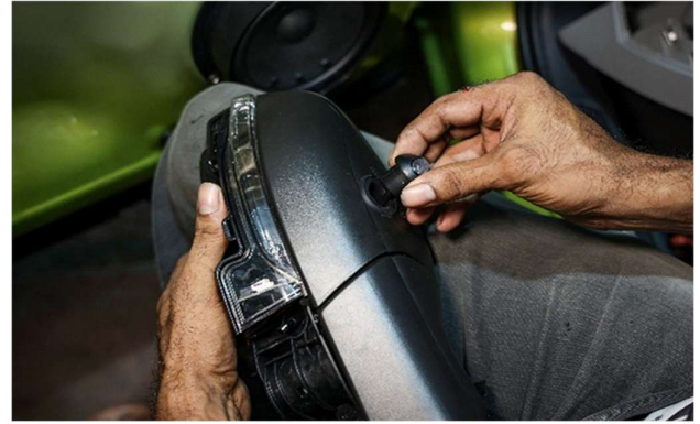
STEP 36 :- INSERT LEFT AND RIGHT CAMERA IN ORVMs RESPECTIVELY WITH RUBBER COVER/CAP ON THE CAMERA.
