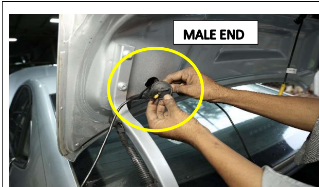
STEP 65 :- ROUTE EXTENTION CABLE YELLOW (PART 4) MALE END AS SHOWN FROM HOLES IN TAIL GATE.
