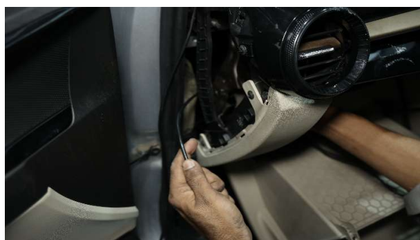
STEP 76 :- BRING CABLE NEAR THE GLOVEBOX AREA FOR NEXT CONNECTIONS.
