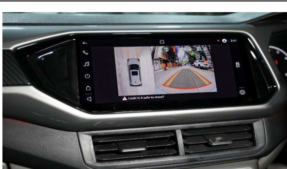
STEP 15 :- FUNCTION CHECK ALL THE CAMERAS HAVE POWER ON INFOTAINMENT.
