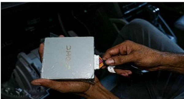
STEP 27 :-CONNECT THE OTHER END OF 32 PIN CONTROL CORD (PART 6) TO JUNCTION /ECU BOX (PART 1 ) AS STEP 10
