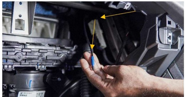
STEP 58 :- PASS THE CABLE TILL THE JUNCTION BOX AREA, JUST LIKE STEP 56
