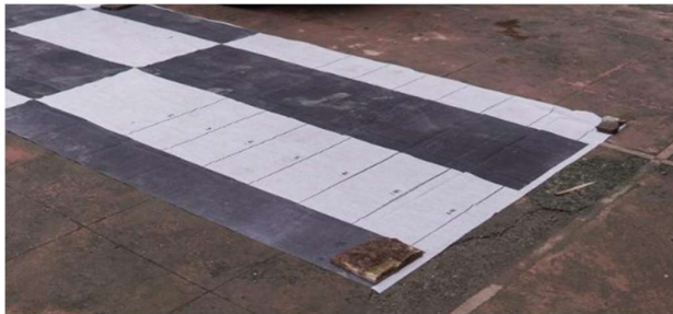
STEP 109 :- OFFSET WILL BE WRITTEN ON THE MAT, PLACE REAR MAT EXACTLY ON 1.0 ON BOTH SIDES, THE REAR MAT SHOULD BE PLACED PARALLELLY TO THE CAR.
