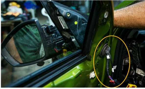
STEP 41 :- CONNECT THE LEFT AND RIGHT ORVM's AND ROUTE CABLES AS SHOWN.
