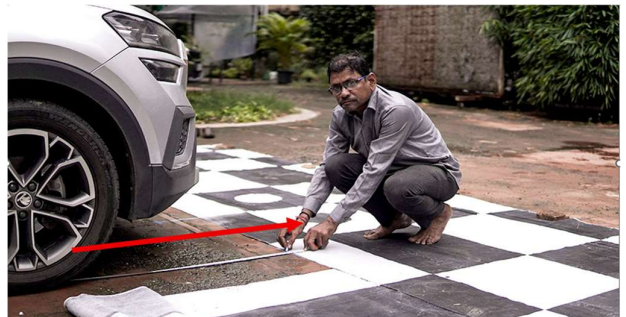
STEP 106 :- MEASURE FROM THE TYRE 35 INCHES AND ALIGN THE MAT 35 INCHES FROM THE BOTH FRONT TYRES. MAT HAS TO BE PLACED. (PLEASE REFER TO THE VIDEO FOR REFERENCE).
